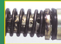
Harmful deposits and varnish build-up—resulting from worn-out, oxidized brake fluid—are apparent on this brake master cylinder piston assembly.
