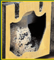
Severe corrosion which can occur when additives that protect the cooling system have been depleted.
