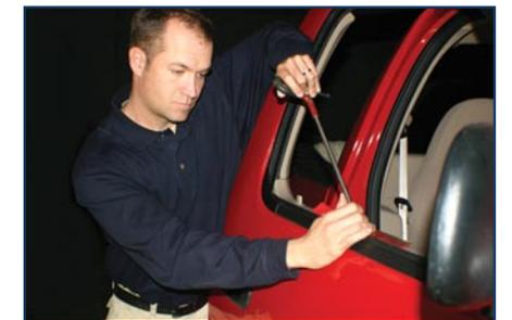
PDR works from behind the vehicle's damage; therefore, it does not require sanding, painting, or body fillers.
